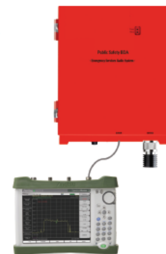
Figure 22.12.1 Measuring UL Noise Power from BDA
